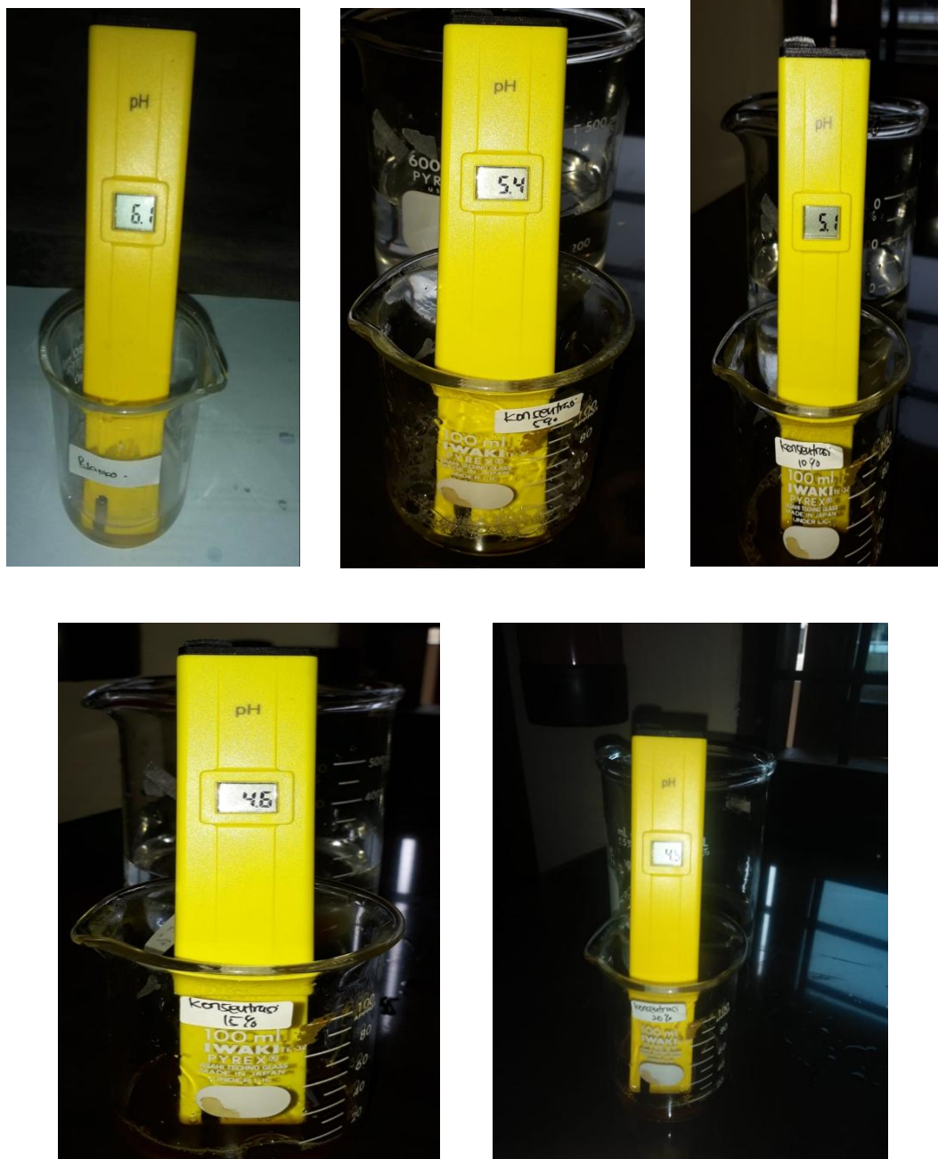
Gambar 11. Ket : Uji pH Sampo Blanko (a), pH 5% (b), pH10% (c), pH15% (d), pH 20 (e).
