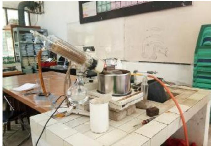
Alat Rotary Evaporator
