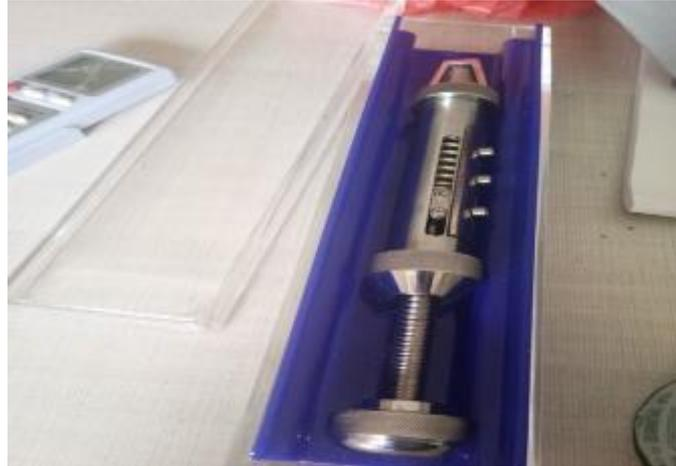
Alat Uji Kekerasan Tablet
